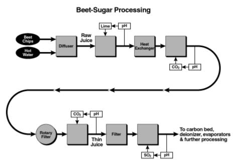
The processing to accomplish this is heavily dependent on reliable pH measurement and control as illustrated in the accompanying figure. Described are the early stages of treatment for the manufacture of beet sugar. Cane sugar processing uses many of the same operations.
