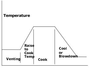
Time Figure 1—Retort Time/Temperature Cycle
