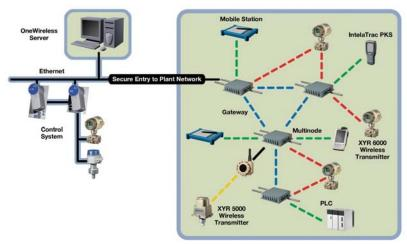
A wireless mesh network has multiple paths between access points, or nodes, to establish a redundant infrastructure.
