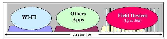
Efficient wireless mesh networks mitigate signal interference in these limited ISM bands by employing a frequency-hopping spread spectrum (FHSS). This technique modulates the data signal with a carrier signal that periodically "hops" from frequency to frequency across a wide band. Through the relaying process, a packet of wireless data will find its way to its destination, passing through intermediate nodes with reliable communication links.
